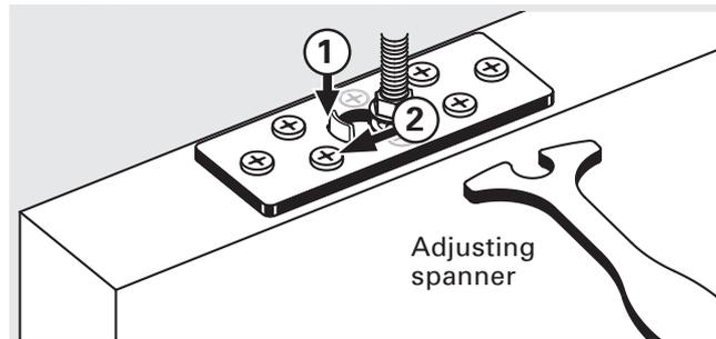
It is not always easy to slide the spanner sideways. You may need to relieve the door's weight by putting a wedge between door and floor.
